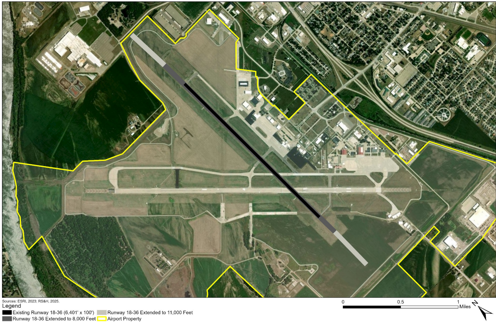
Figure 2-6 Alternative 4: Runway 18-36 Extension
