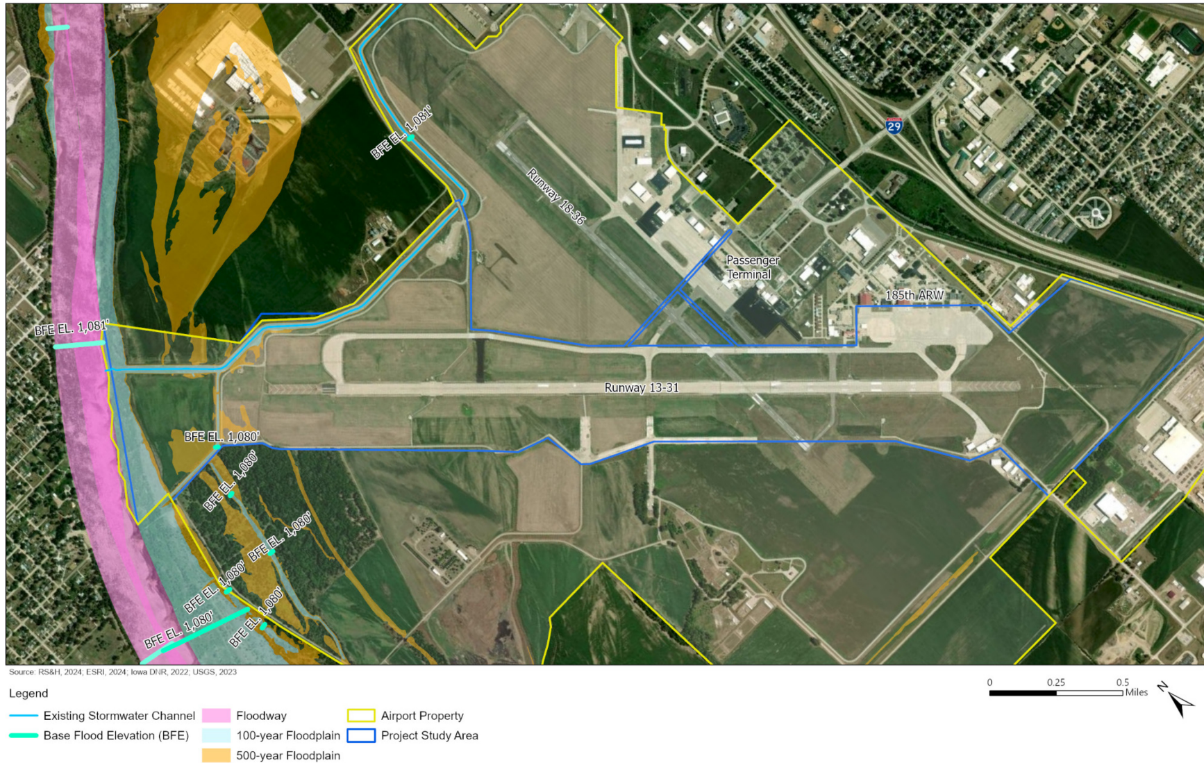
Figure 3-15 Existing Floodplain Conditions
