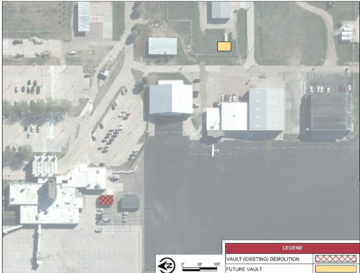
Figure 4-24 Electrical Vault Relocation
