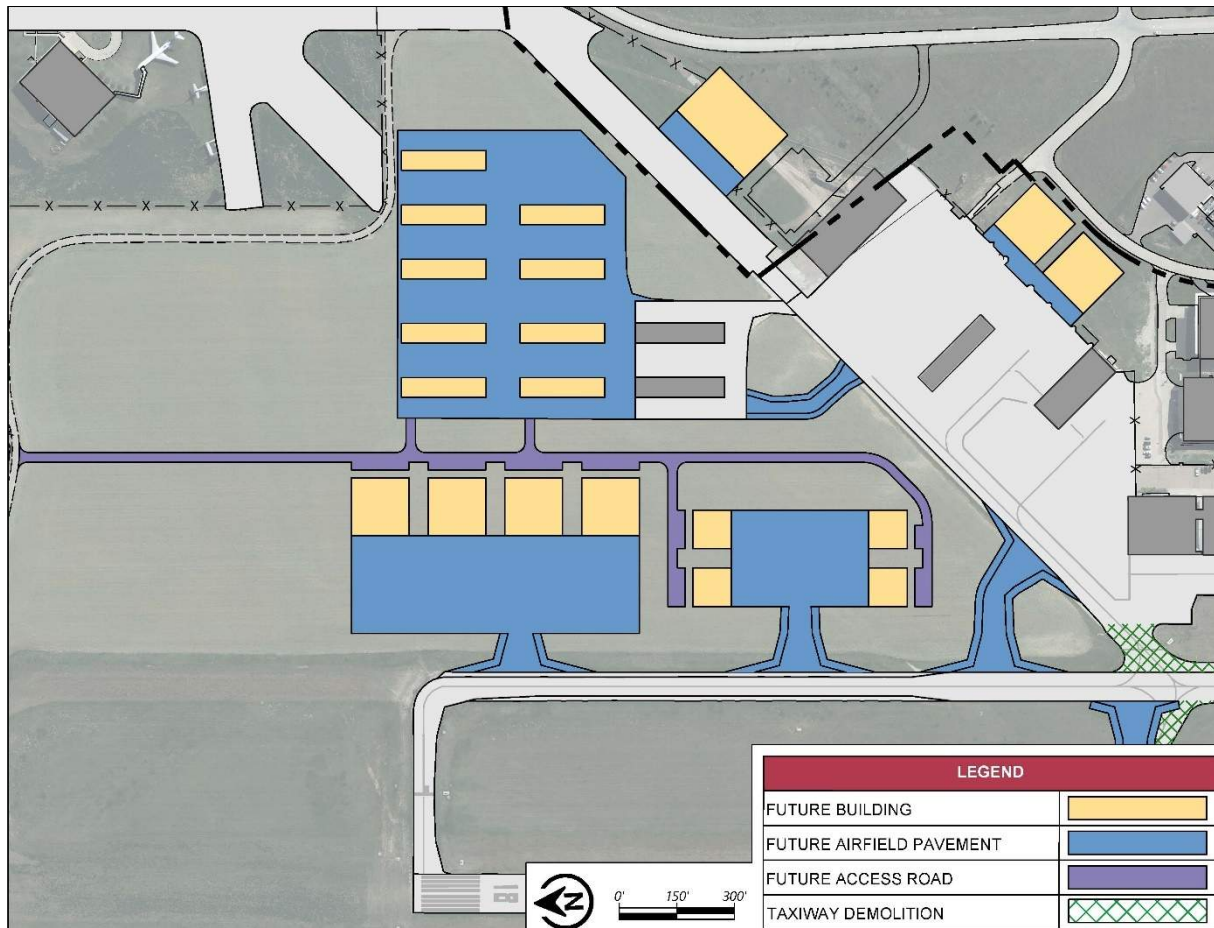
Figure 4-25 General Aviation Hangar Development Plan (North Airfield)
